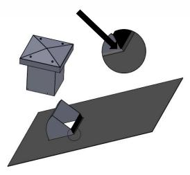
For extra protection against water it is recommended to apply a mastic seal between the bottom part of the ventilation cowl and the roof surface. When installing the cowl pipe, press it down into the mastic seal on the rear side (the low side) of the bottom part, and then secure it on both sides with the included mounting screws (x4).
