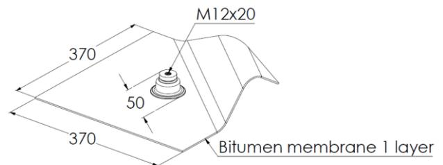
Roof console 2 layers bitumen membrane
