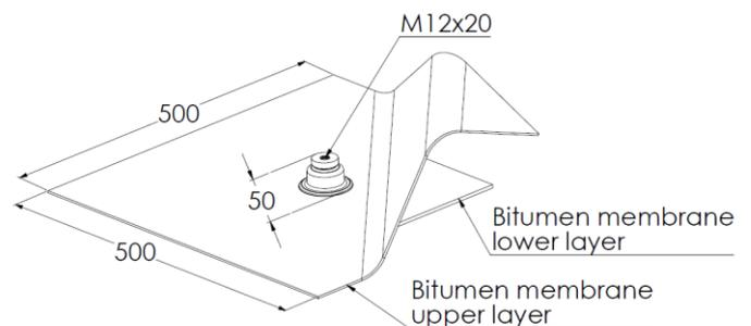
Roof console 1 layer roofing foil
