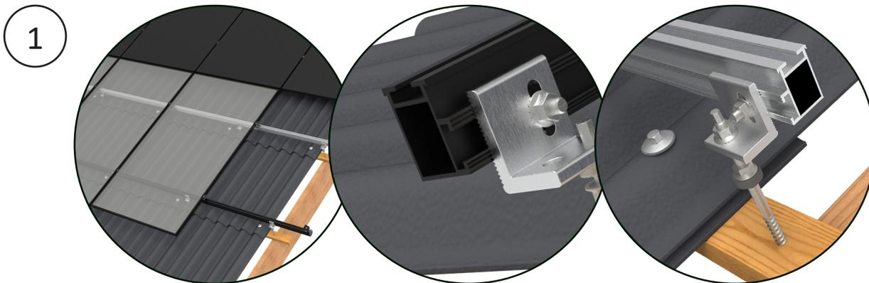
The first profile, which is oriented down towards the eaves, may be visible. In cases where a visually uniform finish is desired, the first profile can be chosen mounted on the underside of the hanger bolt, so that the upper part of the hanger bolt is not visible. Different anodized profiles can also be selected, so that the profiles can have the same colour as the panels.
