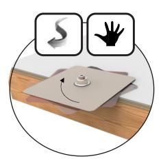
With the pre-assembled Console Adapter installed the Console is simply mounted by engaging the M12 thread of the Console Adapter with to the upstanding Hangerbolt.
