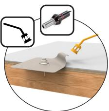
Once the Console has been brought to the intended position in good contact with the general roofing surface and with its perimeter edges correctly aligned, the membrane of the console is either torched or welded to the existing
