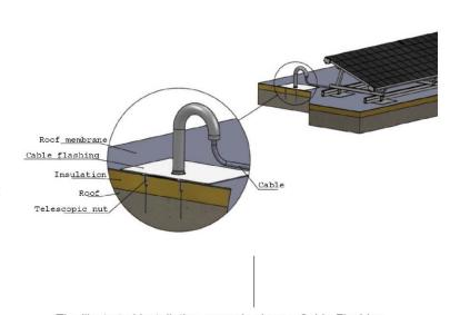
The illustrated installation example show a Cable Flashing mounted on a flat roof solar cell installation.
