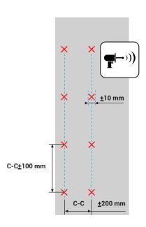
The illustration above shows the generally allowed tolerances for positioning of Roof Consoles. If larger deviations are needed, Fixnordic must be contacted.
