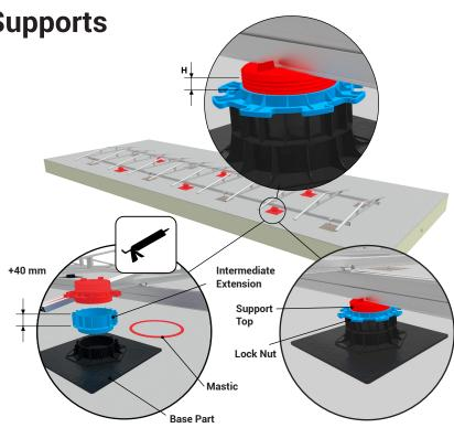
This illustration shows the components of one Intermediate Support.
