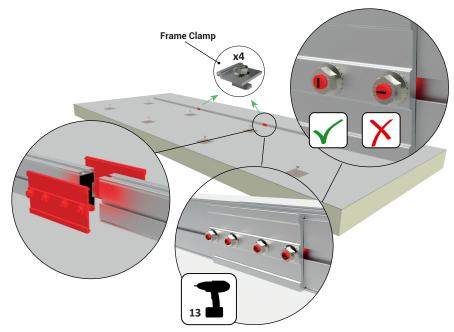
This illustration showns how the two Assembly Brackets are positioned in each profile assembly point. As the hammer-head bolts are tightened, they must rotate 90° to secure correct strength of the assembly. Please note that each bolt has a marking at it's end that shows the position of the hammer-head bolt.
