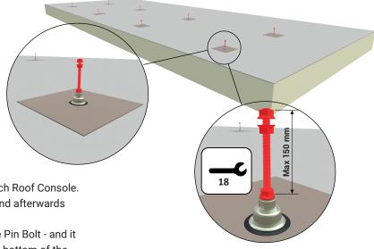
The Pin Bolt is installed into the internal M12 thread of each Roof Console. It must be inserted approximately 20 mm into the thread and afterwards secured with the bott om lock nut.
