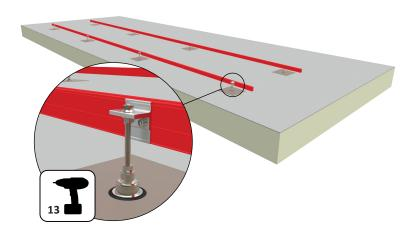
Installation of the assembled Carriage Profiles is done in the same way as the assembly of the Carriage Profiles - i.e. by using the pre-installed hammer-head bolts to secure the assembly. Again, it is very important to pay close attention to the position of the hammer-head bolts.
