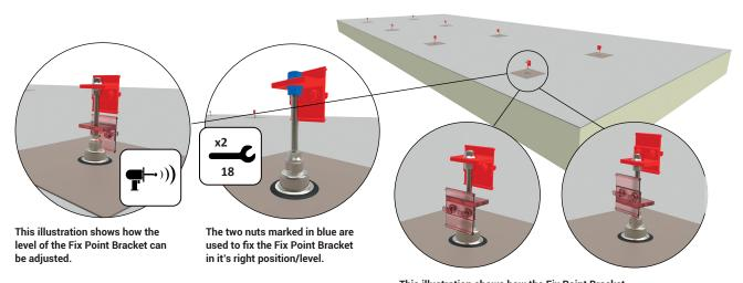
Before installing the Fix Point Brackets, the level of the Module mus be determined. Normally, this is done by locating the highest point of the roof surface which is the point defining the minimum distance between the Module and the roof surface.
