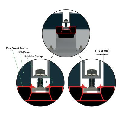
When the distance (D) is determined, it is important to note that this distance should include extra distance to accomodate tolerance on the used PV-panels. This tolerance can be both on length/height but also 'straightness' of the panels might diff er from panel to panel.
