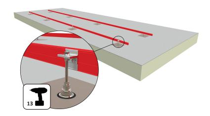
Installation of the assembled Carriage Profiles is done in the same way as the assembly of the Carriage Profiles - i.e. by using the pre-installed hammer-head bolts to secure the assembly. Again, it is very important to pay close attention to the position of the hammer-head bolts.
