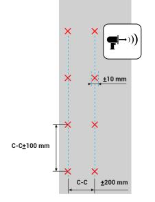
Positioning of Roof Consoles depends on each individual project and the size of the given module. Specific module dimensions are defined in the corresponding Technical Design Report created by Fixnordic system compliance.
