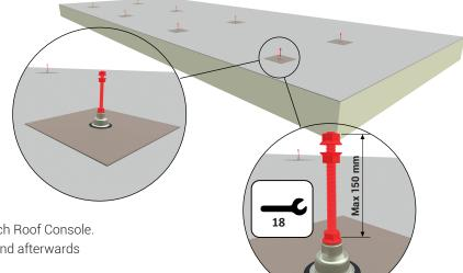
The Pin Bolt is installed into the internal M12 thread of each Roof Console. It must be inserted approximately 20 mm into the thread and afterwards secured with the bott om lock nut.
