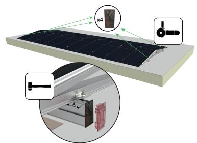
The illustration above shows the installation of the End Cover.
