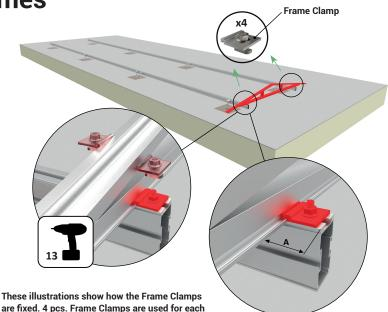
These illustrations show how the Frame Clamps are fixed. 4 pcs. Frame Clamps are used for each Frame. The min. distance (A) from the end of the Carriage Profile to the first Frame must is 35 mm.
